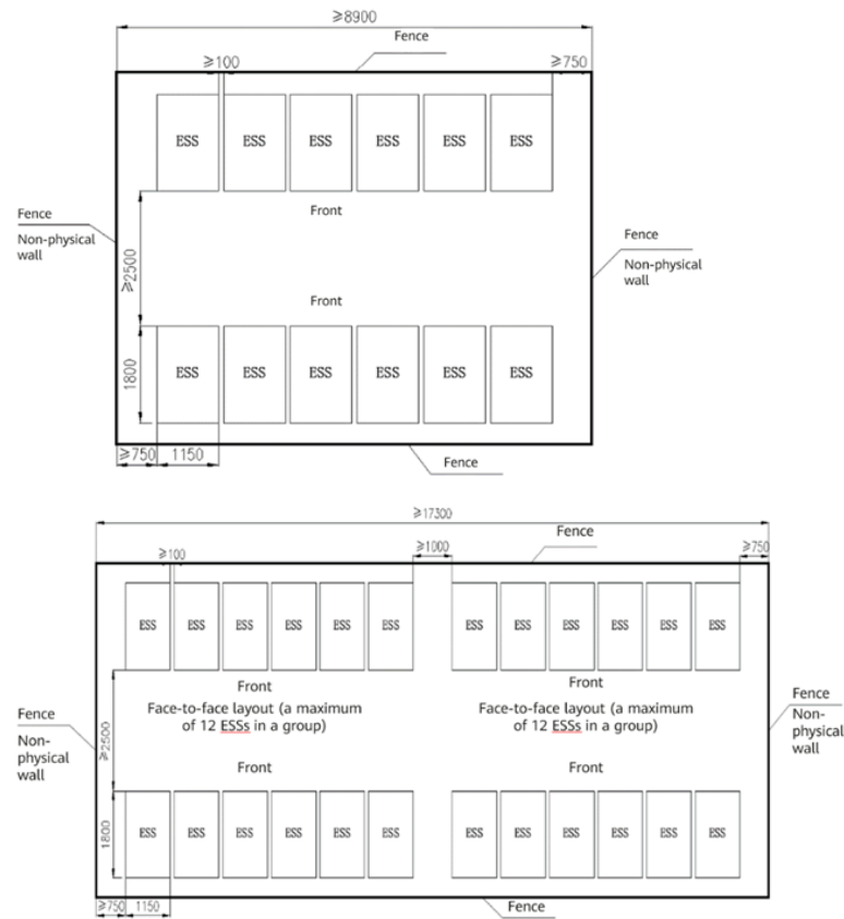
Figure 4-6 Typical array layout (dual-row face-to-face)
