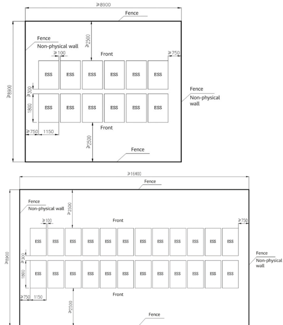
Figure 4-5 Typical array layout (dual-row back-to-back)
